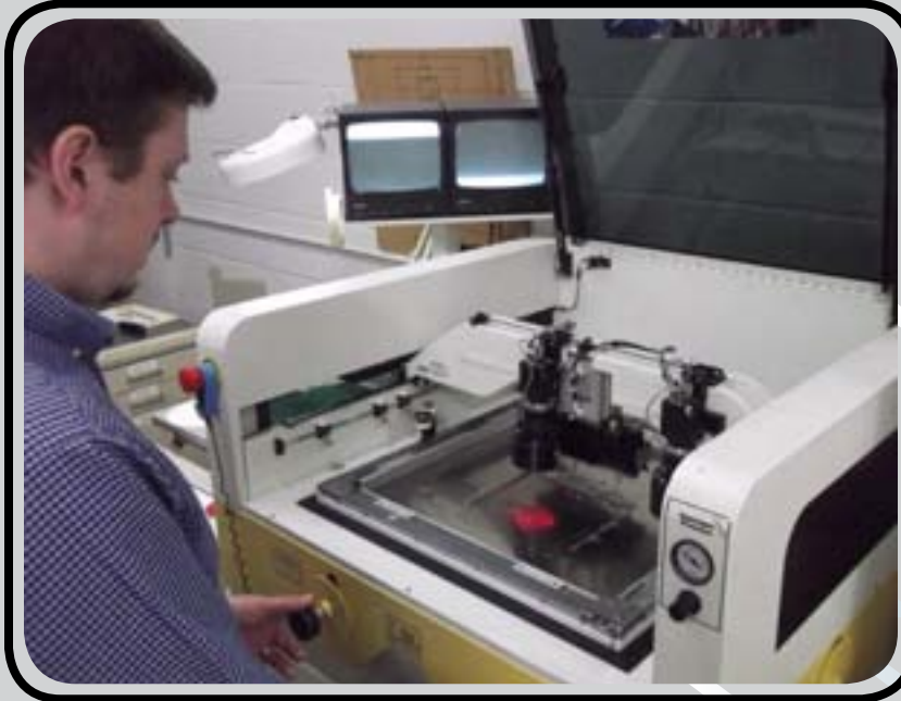
Stencil Printing of Solder paste and Adhesives is done by full automation to ensure accuracy and repeatability.
