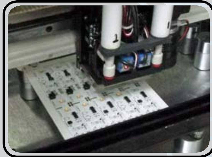
Pick and Place of surface mount components accomplished by precision, high speed robotics.
