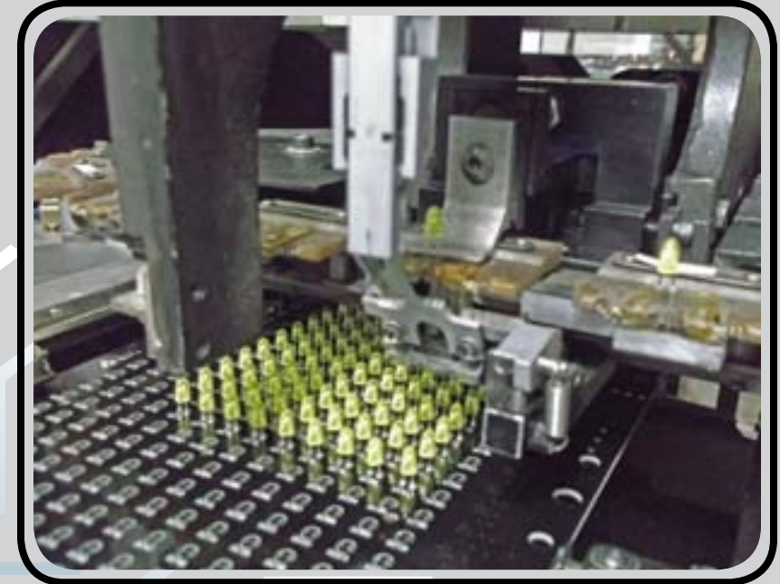
Thru-Hole components are installed on Radial and Axial insertion machines or by hand as required.
